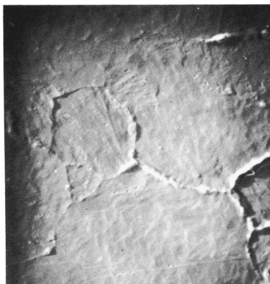
FIG. 2. Electron micrograph of a wavy silver surface. Scale: 1 cm = 6500 Å.
